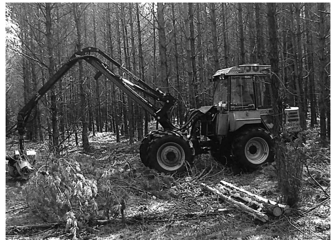
Figure 2. Harvester Vimek 404 T5 during bucking of assortments
