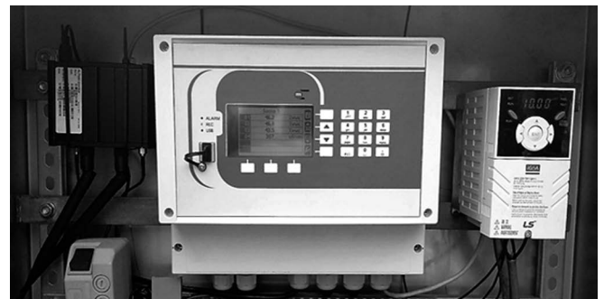
Figure 2. MPI-DN multichannel electronic recorder (middle) network connection router (left) and wave modulator for irrigation system (right) at research field in Nędza nursery farm (photo G. Durlo)
